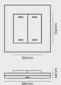
Powered by EnOcean's energy harvesting technology, each press of the switch generates enough energy to send a radio signal to a relay for a totally wireless and battery-free solution.
