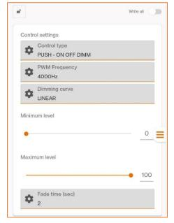
**Control type**: allows you to set the operating logic of the analog input in case of connection to a button or switch.
