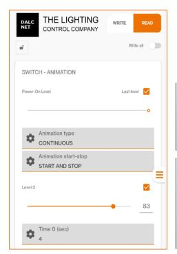
**Power On level: it** is the intensity value to which the output is brought as soon as the device is powered if the switch is on ON. If the switch is OFF (open) the light will remain off.
