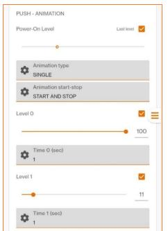
**Power On level:** is the intensity value to which the output is brought as soon as the device is powered
